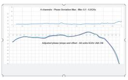
During Q1 of this year, we have released a new phase-matched multichannel RFoF subsystem. The system is provided as a complete end-to-end RFoF product. This subsystem with 6 RFoF links achieves better than  $\pm$  6° of full band phase. We are currently streamlining the production operations of these kinds of phase-matched systems by automating measurement and production testing.
